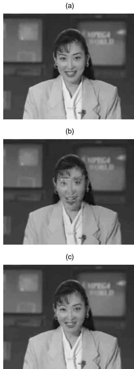
Figure 5-8: Comparison of a frame of “Akiyo”. (a) shows the reconstructed frame with no channel errors, and (b) and (c) show the reconstructed frame after transmission through a simulated GSM channel with 4% BER using (b) EEP coding and (c) UEP coding. UEP produces visibly better images than EEP for the same amount of channel-coding overhead.
